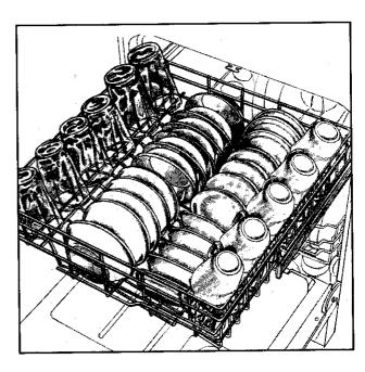
The upper rack may be removed if desired. Push inward on the front of the rack rail ends to unsnap. Remove rail ends and pull out rack.
